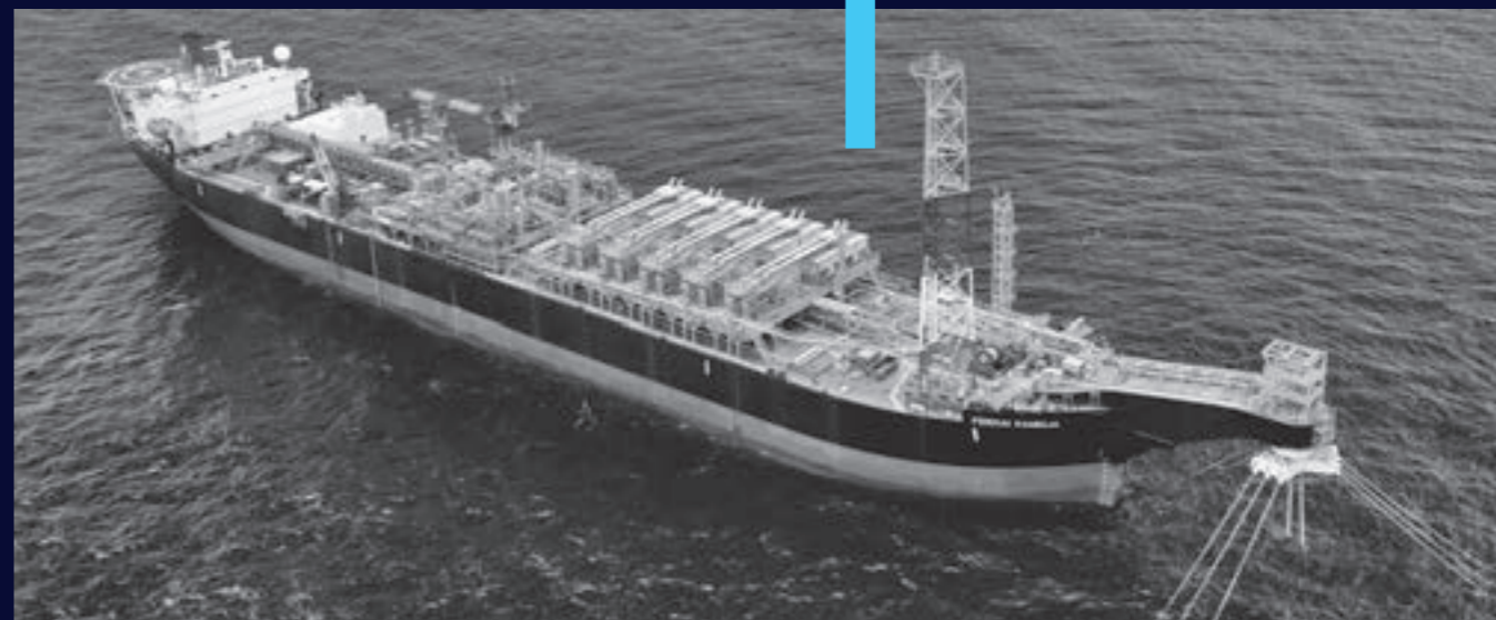
ABOVE: PERISAI KAMELIA FPSO EXTERNAL CANTILEVER TURRET AND SWIVEL STACK
